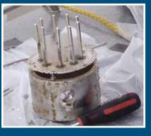
PMDs (Polyethylene Membrane Devices): pick up dissolved oil and gas related chemicals (hydrocarbons). They are passive samplers that stay in the water for one month. They are changed up to four times per field season. The University of Alberta does the analysis.
