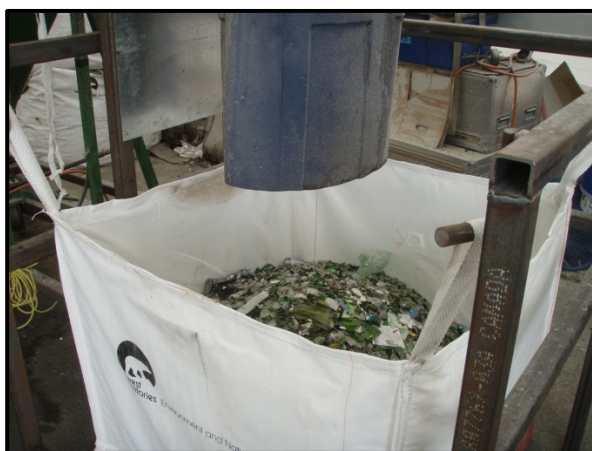
The Yellowknife processing centre breaks glass into specially designed bags.
