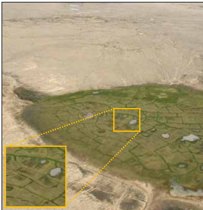
Figure 8. Low-centre polygons are indicative of continuous permafrost in wet terrain (e.g., drained lakes, within which these have developed). Ice wedges develop in cracks, pushing up soil ridges adjacent to the wedges and creating dams that trap water inside the resulting polygons. High-rimmed ridges surrounding wet shallow central pools of water are distinguishing features. Location: East Banks Hills MA Ecoregion.
