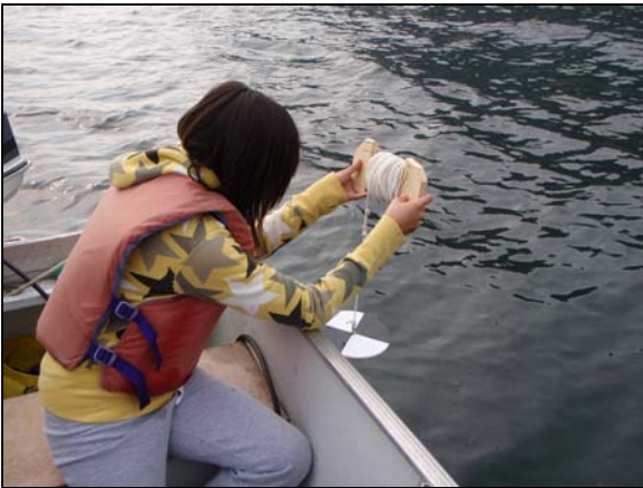
A student using a Secchi Disc to measure water clarity
