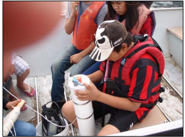
A student using a water sampler to collect water at different levels in the lake
