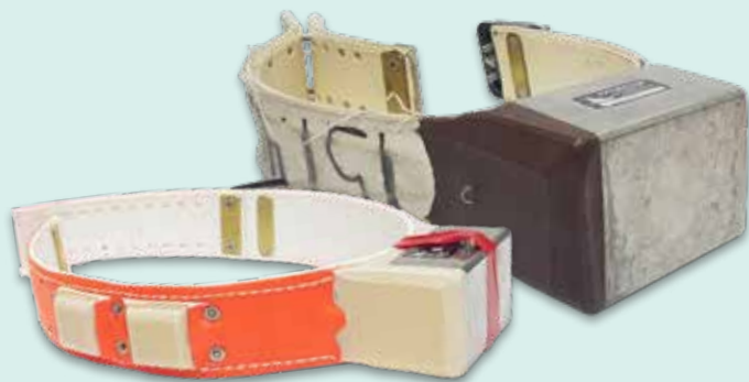
New collar, left, weighs about a third less than older collar, right, due to a smaller, lighter battery
