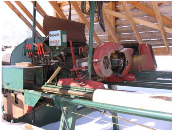
Figure A 2 Old Log Lathe Used To Produce Log Packages at Jean Marie River
