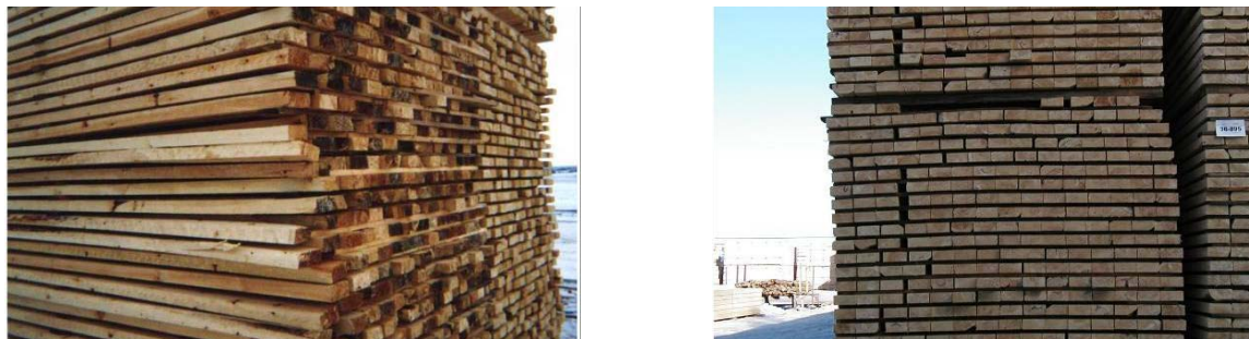
Figure 25. Example of Poor Sticker Alignment (L) and Poor Stacking (R).
