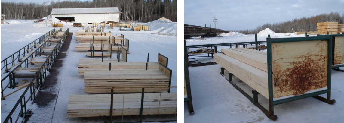
Figure 21. “Live Chain” (L) and Detail View of The Sorted Lumber Pile in The Buggy (R).
