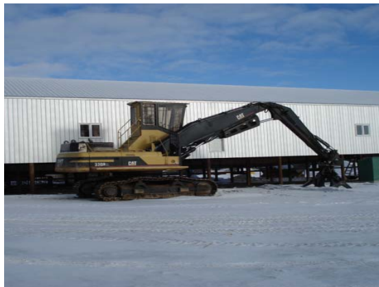
Figure 16. Cat 330 for Unloading Logs from the Truck (L) and Portable Slasher (R).
