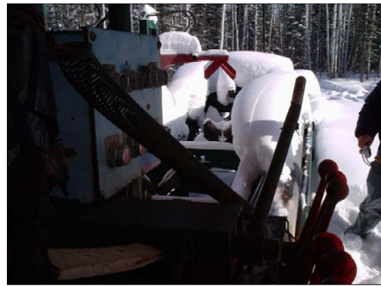
Figure A 2 Old Log Lathe Used To Produce Log Packages at Jean Marie River
