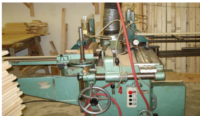
Figure 9. Modified Industrial Shaper Used as End-Tenoner
