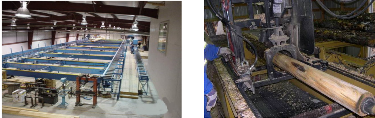
Figure 37. High Production Machine Profiled Log Home Manufacturing Facility (L) and Simple Log Lathe Produced by Isaac Ironworks Ltd., Designed For One-man Operation (R).
