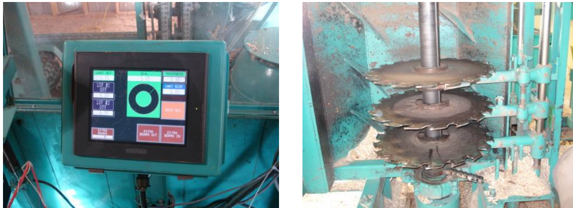
Figure 18. Detail View of Sawyer's Console (L) and Edger With Three Movable Saws (R).
