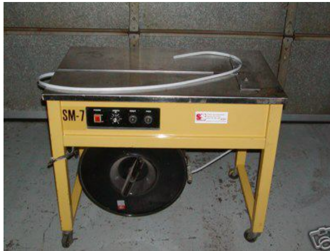
Figure 12. Strapping Machine (L) Used for Strapping Products Into Bundles (R)
