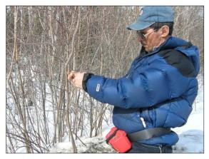
Use hip chain measuring device or pacing to measure off 10 m. to the first trap set. Make sure the counter on the hip chain device is set to "0" before starting.
