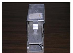
For storage, the tunnel is rotated 90° and inserted into the bedding chamber. To set the trap up, pull the tunnel out, rotate it so the ridges are up, and insert it into the larger chamber.
