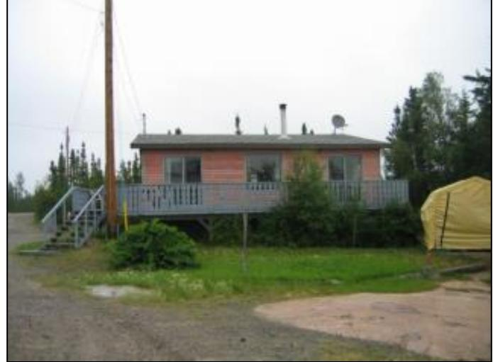
Many structures have combustible debris piles (firewood, lumber, etc) immediately adjacent to the structure, increasing the threat of wildfire to the structure. Open decks and undersides are common.
