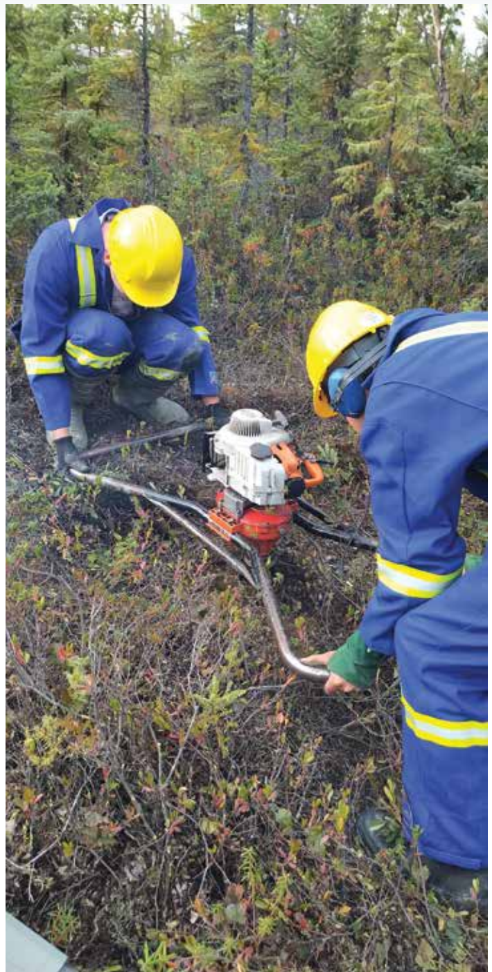
University of Waterloo and Wilfrid Laurier University graduate students collecting shallow cores of permafrost with a portable coring technique in the Central Mackenzie Valley. Photo credit: David Rudolph, University of Waterloo
