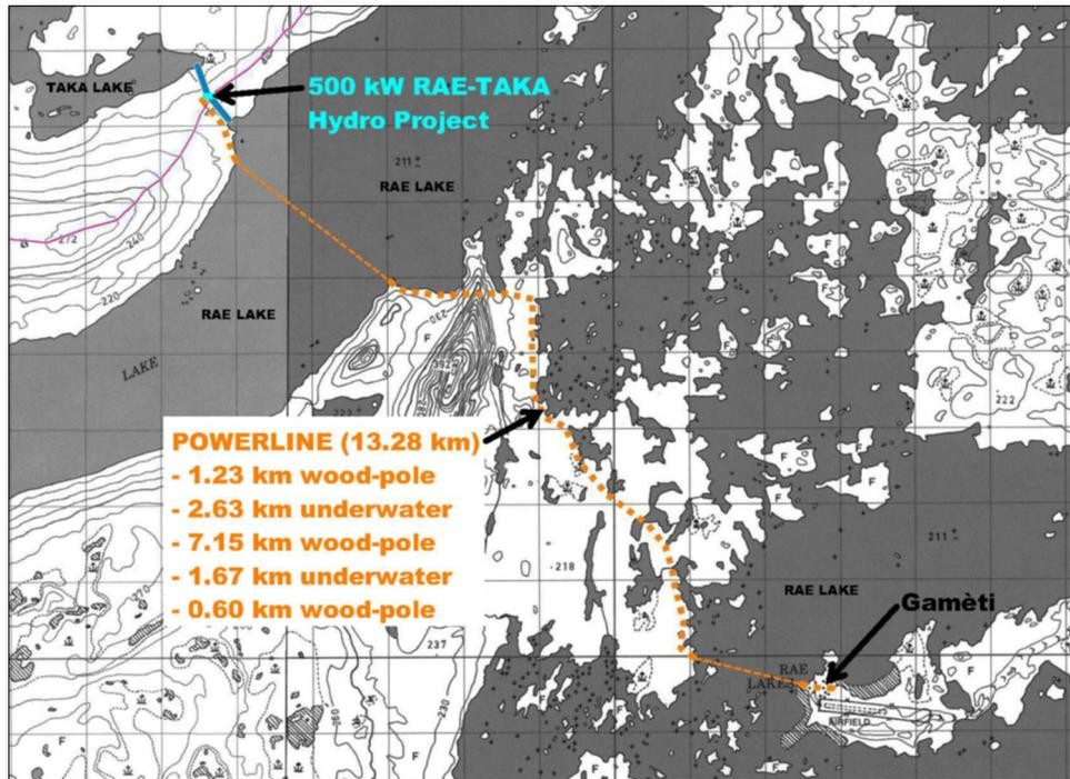
**Figure 26.** Proposed Transmission Line from Taka Lake to Gamèti for the Rae-Taka Hydro Project (PO Sjöman Hydrotech Consulting 2020).
