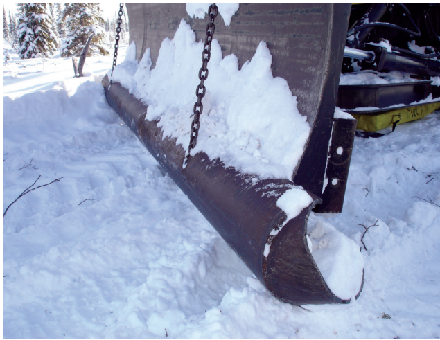
figure 34. A smear blade raises the bulldozer blade off the ground surface.
