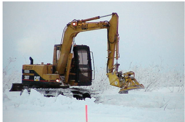
figure 18. A brush cutter can be used to cut and dispose of brush.
