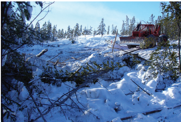
figure 17. Brush can be walked down using a bulldozer.
