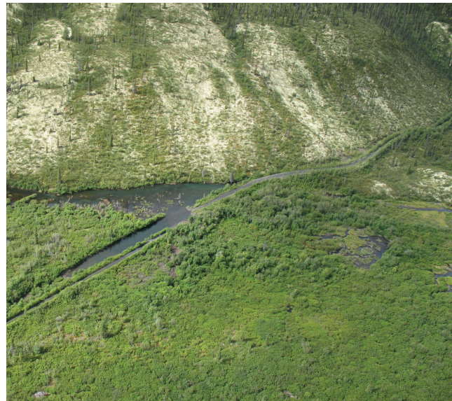
figure 9. Field investigations should be conducted in both the summer and the winter to ensure that the road is built with consideration for the full range of climatic and hydrological conditions.
