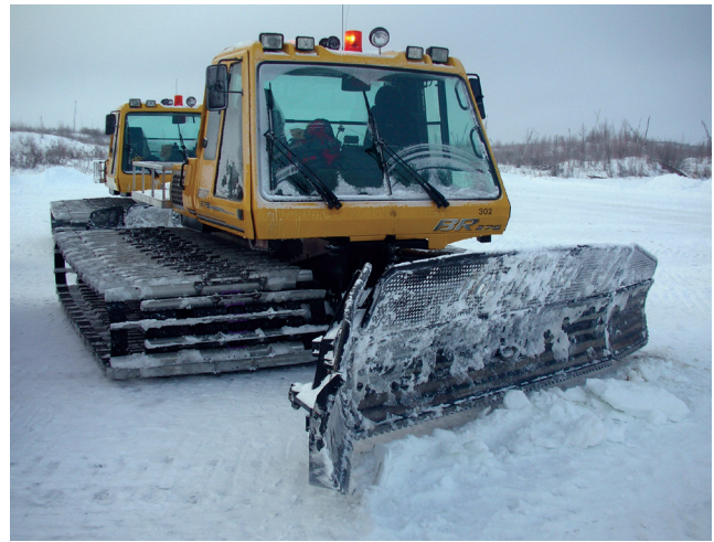
figure 35. A low ground pressure vehicle, such as a snowcat, can be used for a first pass to compact snow on a winter road.
