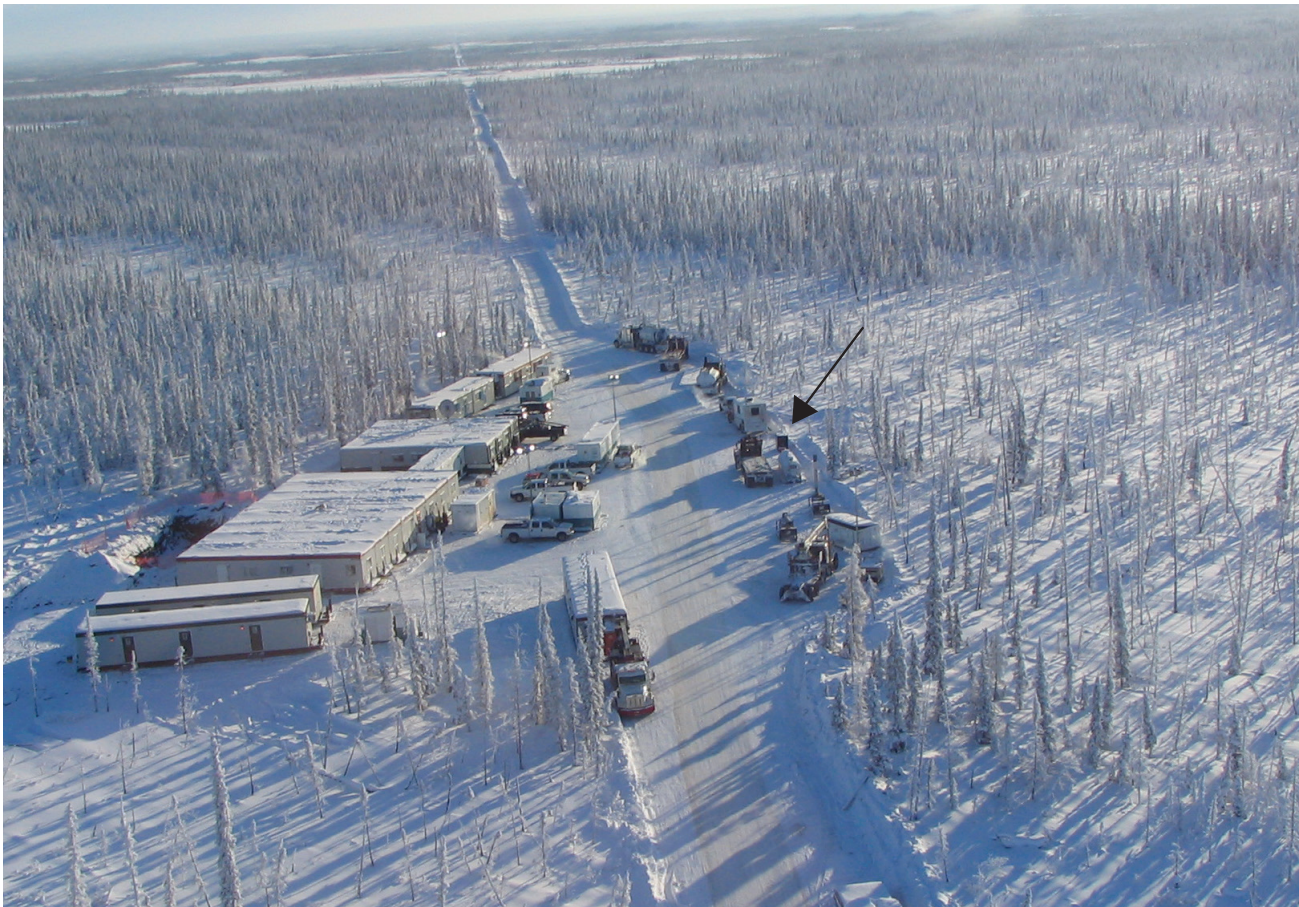
figure 37. Minimal fuel is stored at this mobile camp in a double-walled tank, indicated by the arrow.
