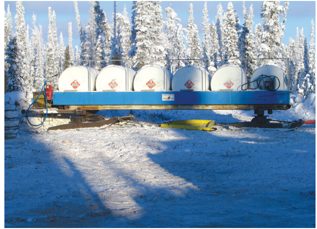
figure 39. A fuel sloop used to transport fuel along seismic lines.
