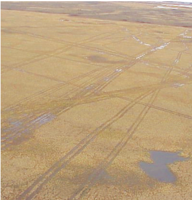
figure 35. Improper use of a seismic line, showing multiple parallel tracks that significantly increased the project's footprint.
