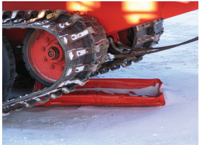
figure 40. Drip trays should be placed under parked equipment to catch unexpected drips or spills.
