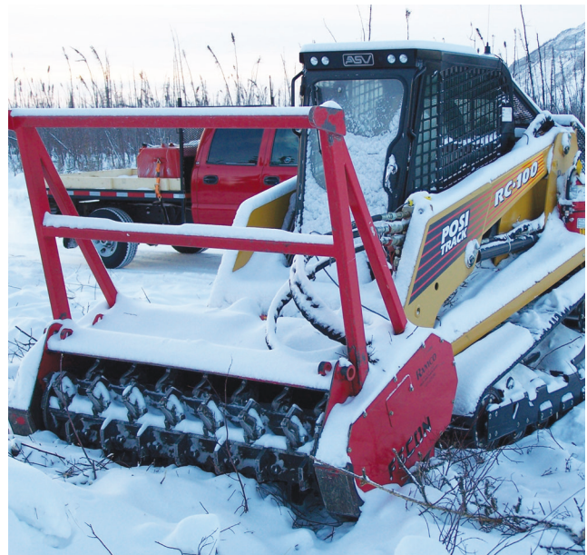
figure 30. A mulcher used for brush disposal.
