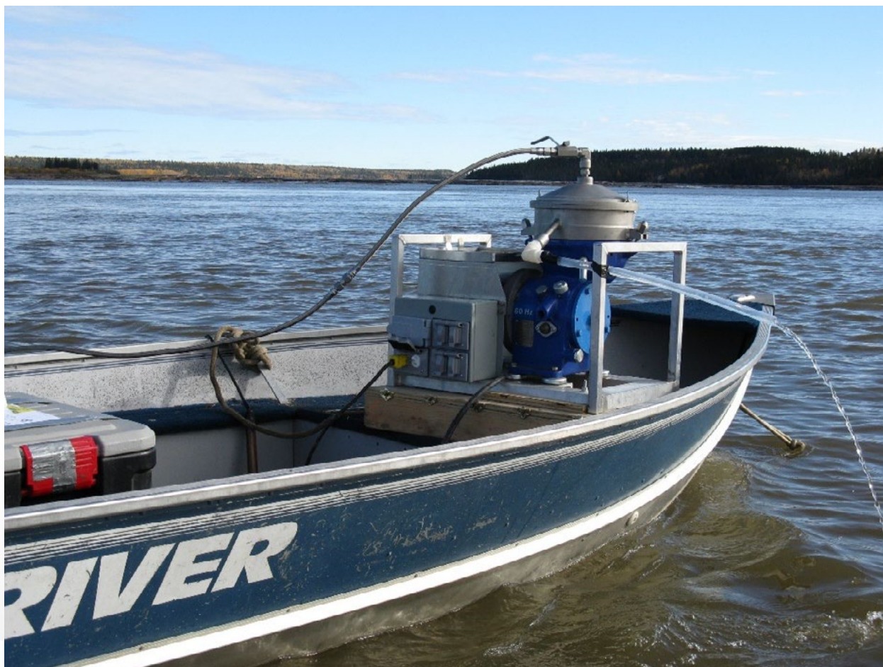
Figure 15. Sampling suspended sediment on the Slave River below Rapids of the Drowned. The centrifuge (pictured here) separates the river water from the suspended sediment in the river.
