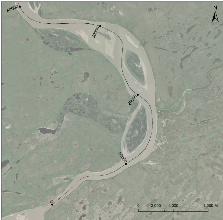
Figure 11-3: River Profile Used to Estimate the Slope of Mackenzie River Near Fort Good Hope
