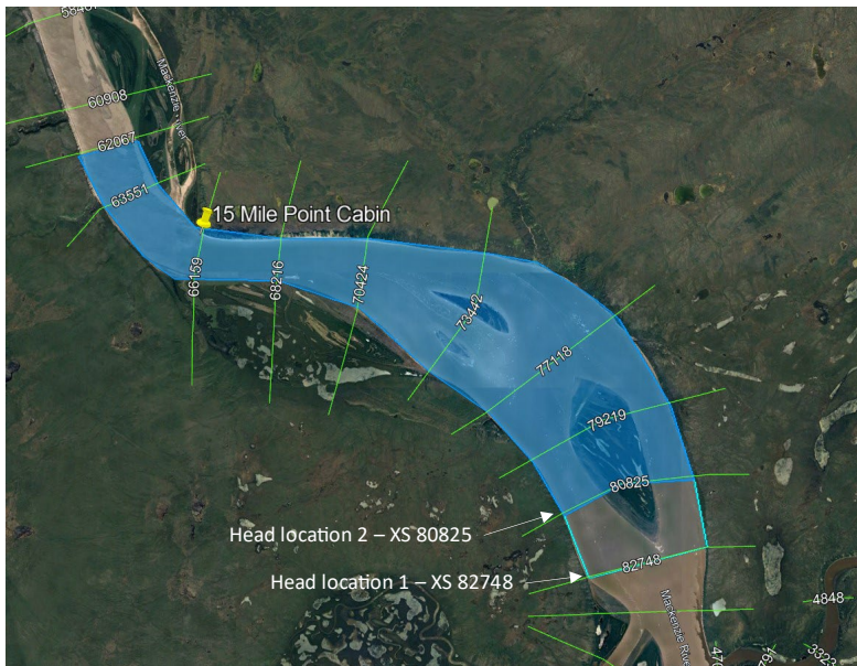
Figure 10-10: Ice Jam Head Locations 1 and 2 considered for Climate Change Scenarios. The blue-marked area represents the maximum ice jam extent for Head Location 2.
