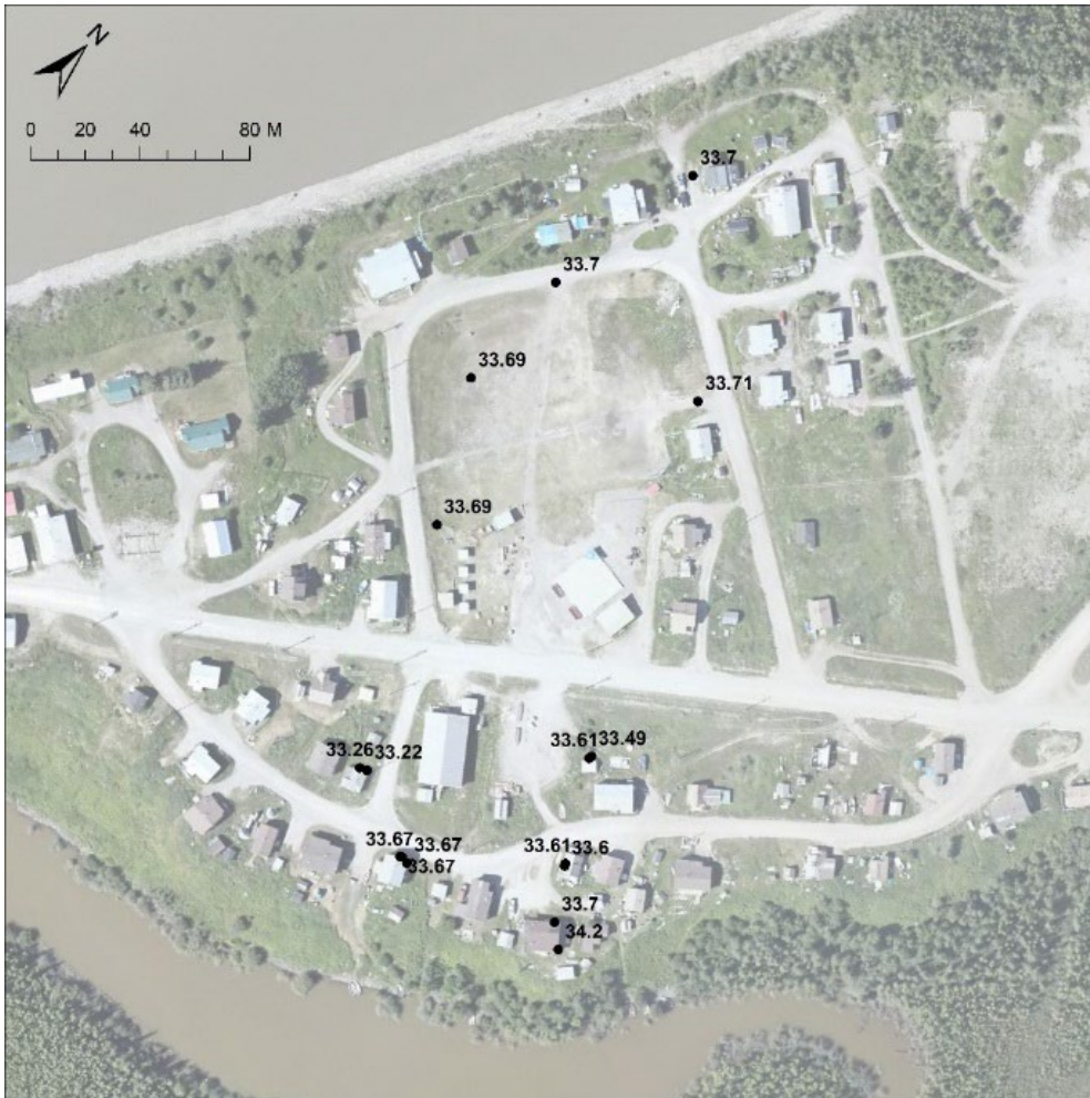
Figure 11-1: May 2021 High Water Marks Surveyed by Ollerhead (2023). Elevations in CGVD2013 datum
