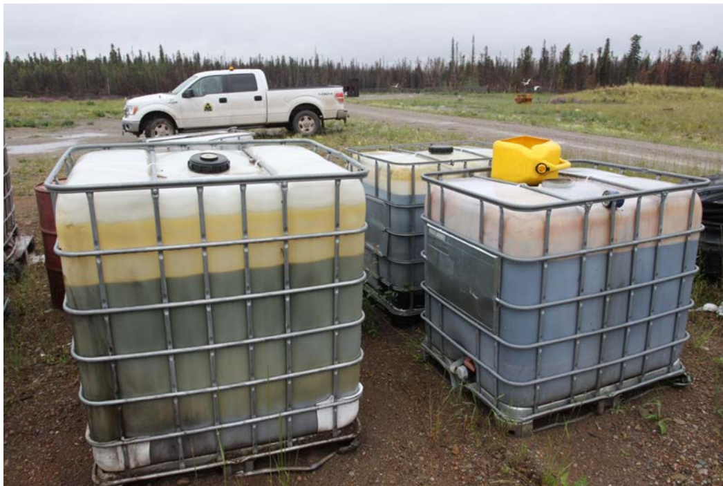
Photo 5: Totes used to Consolidate Hazardous Liquids (Whati)
