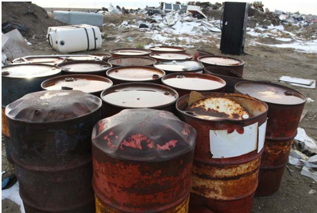
Photo 2: Bulging Drums (Sachs Harbour)
