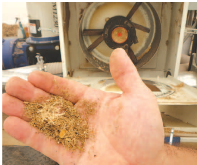
Ground biomass material before pelleting process - Photo Credit: ENR/GNWT
