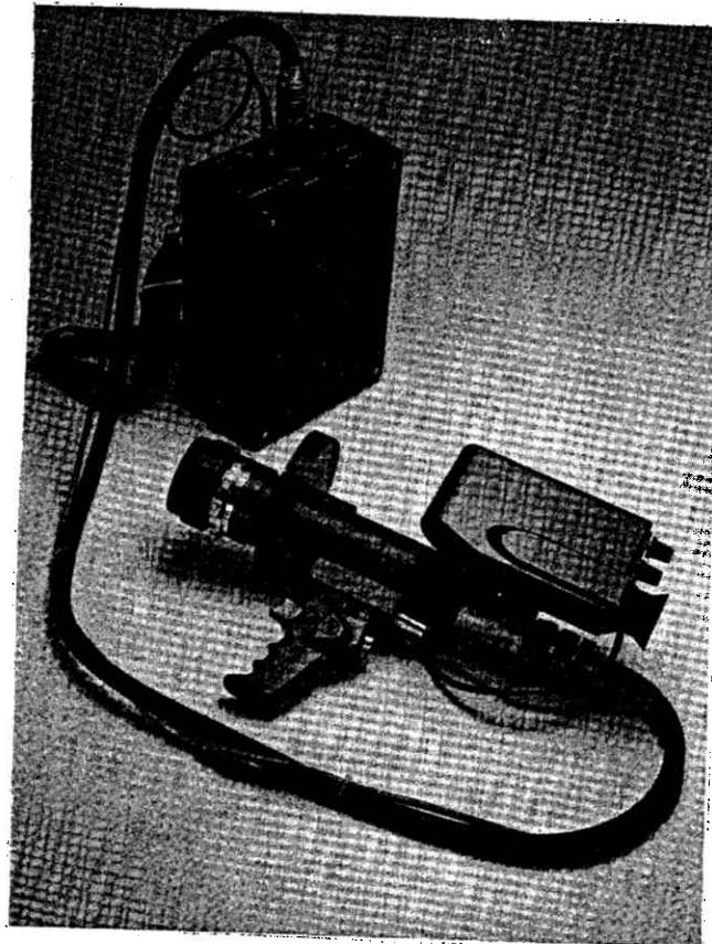
Figure 4. Infra-red detection system used for polar bear detection at Cape Churchill, Manitoba, 1984.
