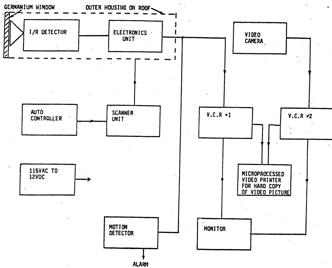
Figure 5. Flow chart of infra-red system used at Cape Churchill, Manitoba, 1984.
