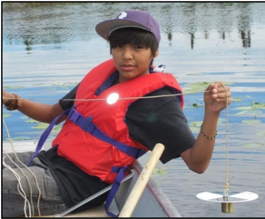
A student using a Secchi Disc to measure water clarity.
