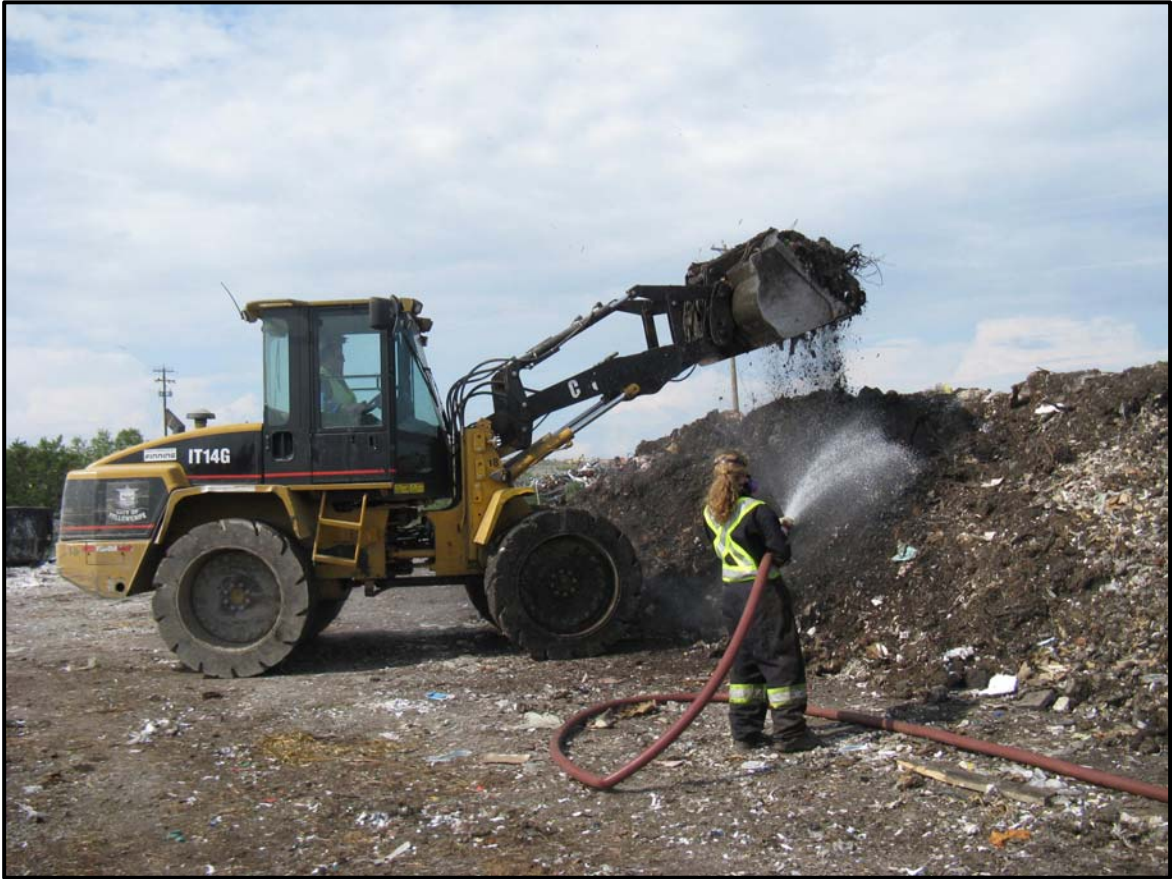
Watering and turning compost windrow (photo courtesy of Shannon Ripley, Ecology North)
