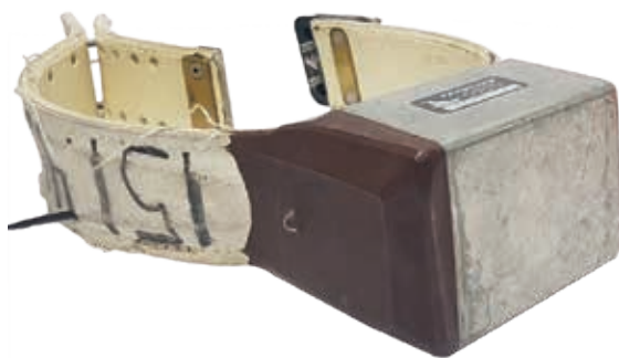
Figure 7. Collars used today (right) are much lighter than the old collars (left) due to a smaller, lighter battery.
