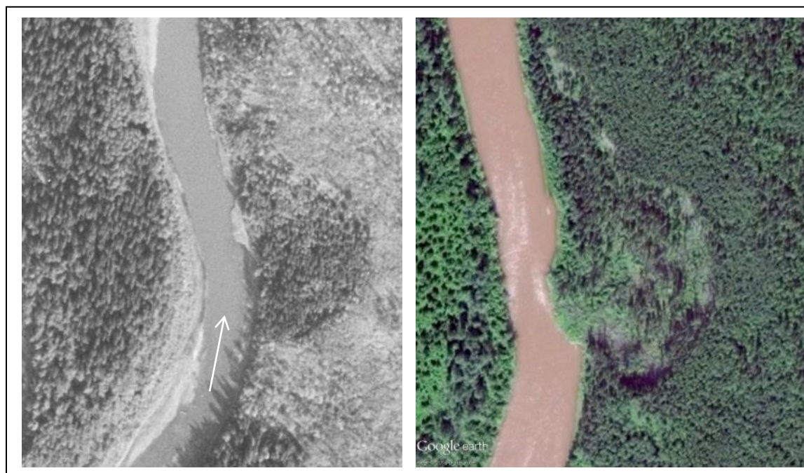
Figure 2-30 Changes in the Channel Morphology in Response to the Reactivation of an Old Landslide at the Hay River near Meander River, Alberta (Site 4)
