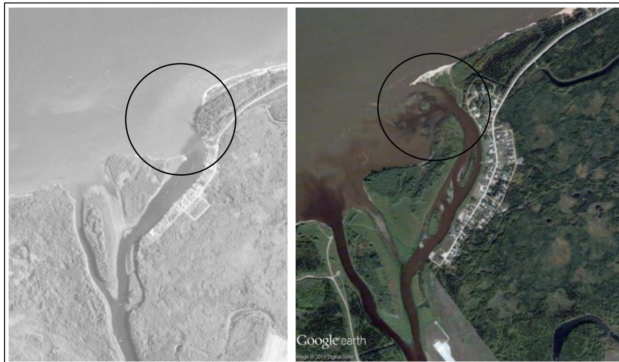
Figure 2-22 Hay River Delta (Site 1) 1955 and 2010 Images Showing Sediment Aggradation at the Mouth of a River Channel on the Northwestern Tip of Vale Island
