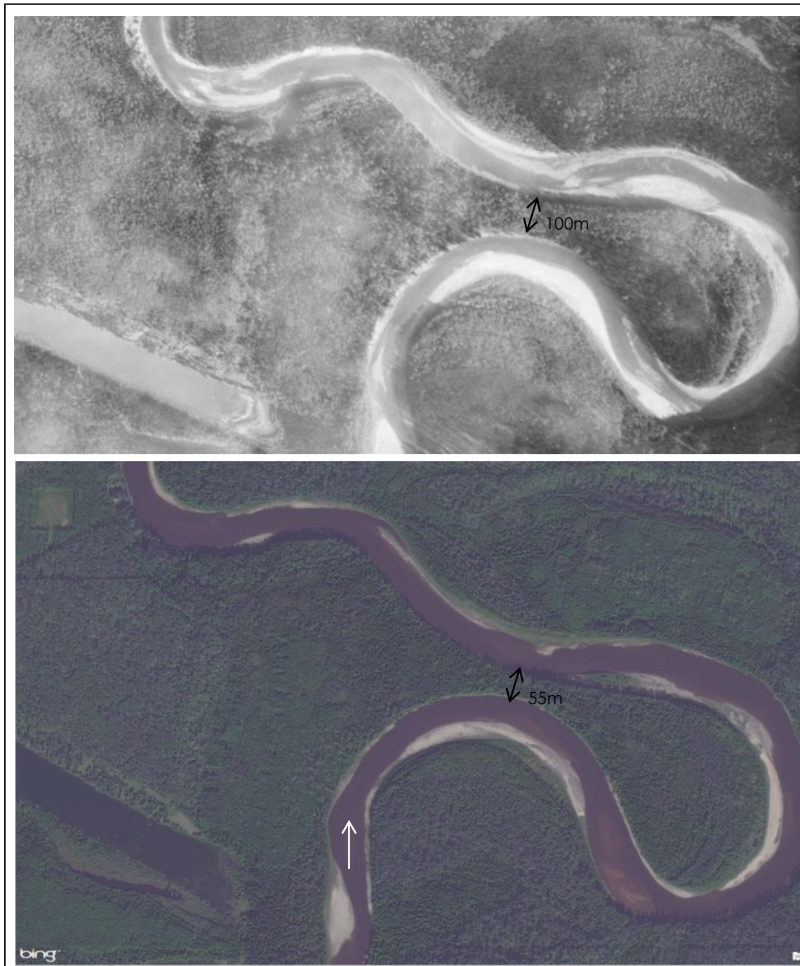
Figure 2-36 Progressive Bank Erosion at the Chinchaga River, near the Alberta Highway 58 (Site 6), that Took Place Between 1955 and 2010
