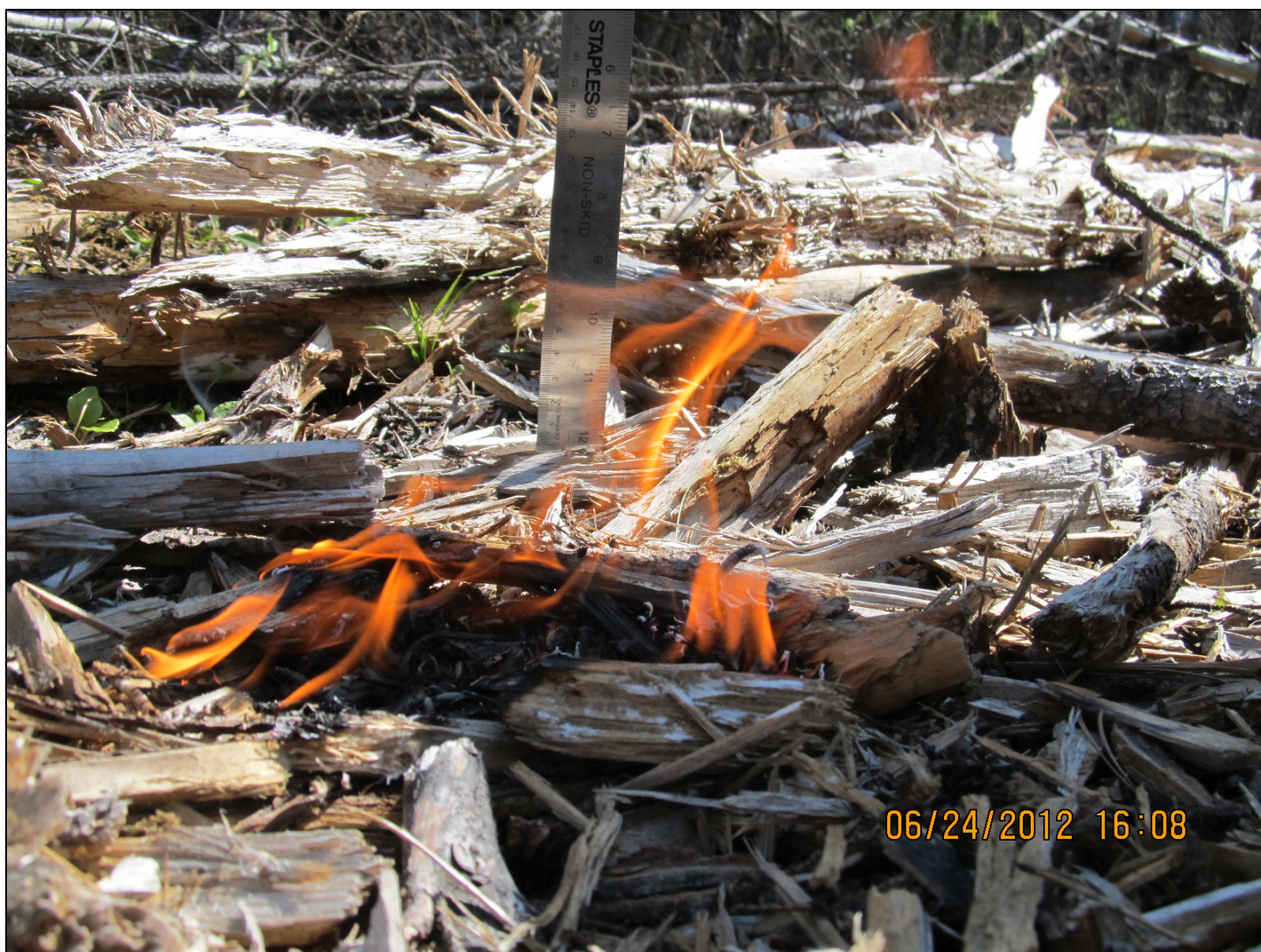
Fire Behaviour in a Mulched Fuel Bed. Photo S Hvenegaard
