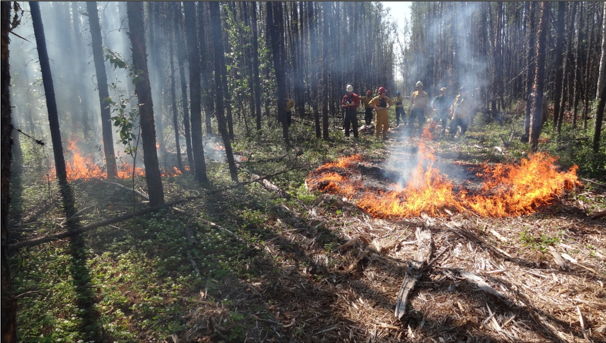
Mulched line and untreated comparison test burn
