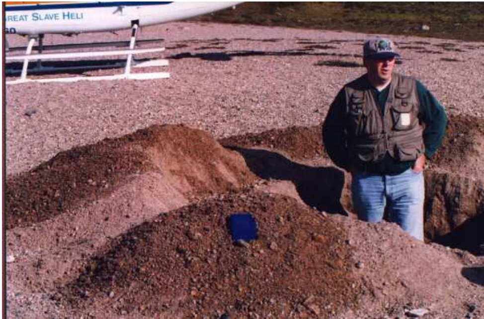
Photo 4: Sample taken from a borehole. The sample is coned and quartered before being sealed for transport.
