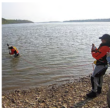
Figure 2. ENR and Smith's Landing First Nation's staff are collecting and processing benthic macroinvertebrate samples through a kick sampling technique in the Slave River.
