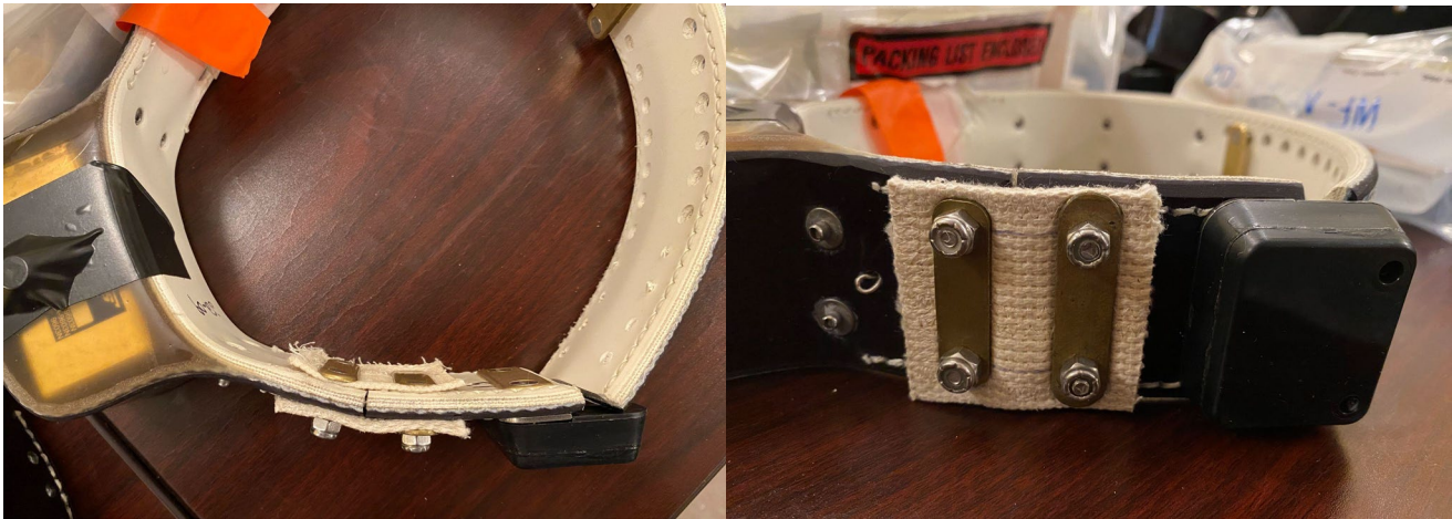
Figure 3. Wolves were fitted with Telonics (Model TGW-4577-4) GPS collars that were designed to lay flush against the neck and contain both a cotton breakaway and a timed-release mechanism (black box). Photo credit: GNWT/A.Wilson, ECC.
