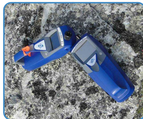
The instruments used to measure the concentration of airborne particulate matter. (Credit: W. Chen)
