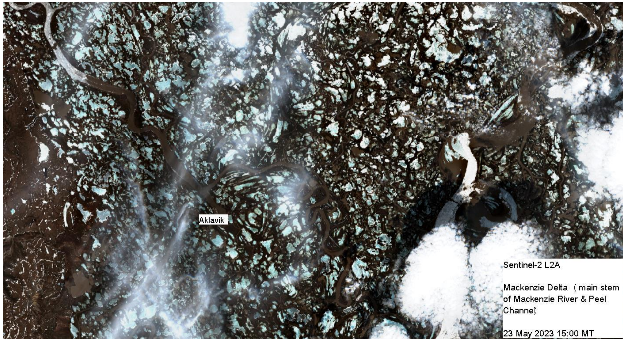
Above – Sentinel-2 L2A imagery over Mackenzie Delta at Aklavik acquired on 23 May 2023 at 15:00. The image shows open water at Aklavik with an ice jam approximately 25 km downstream
