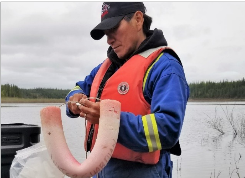
K'ahsho Got'ine Guardian Buddy Gully, prepares a semipermeable polyethylene membrane device (SPMD) to sample water. (Credit: K. Gurney)
