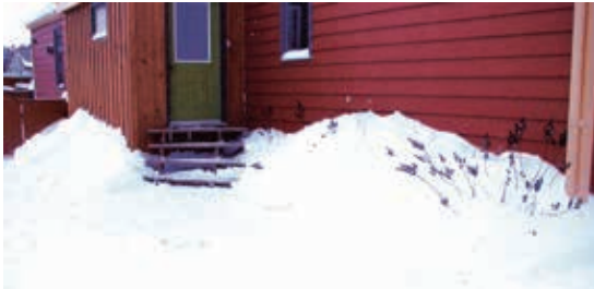
Snowbanks hinder the cold from recharging permafrost during the winter
