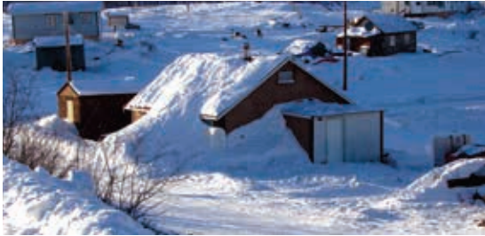
Snowbanks do not allow the cold to recharge permafrost in the winter
