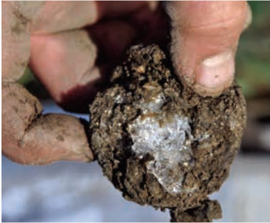
Ice-rich permafrost from a core sample photo by Mike Palmer
